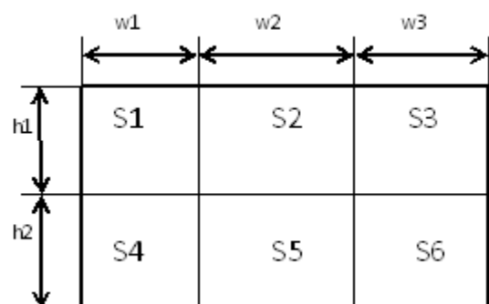
Fig.1 Six segmented rectangular filter. Average pixel value in each segment are computed and compared with each other to find whether they satisfy certain conditions
